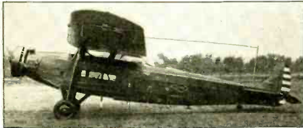
Left—Army plane fitted with new automatic short-wave landing system. A series of vertical short-wave radio-guide beacons, one form of which is shown at the right, are used.
